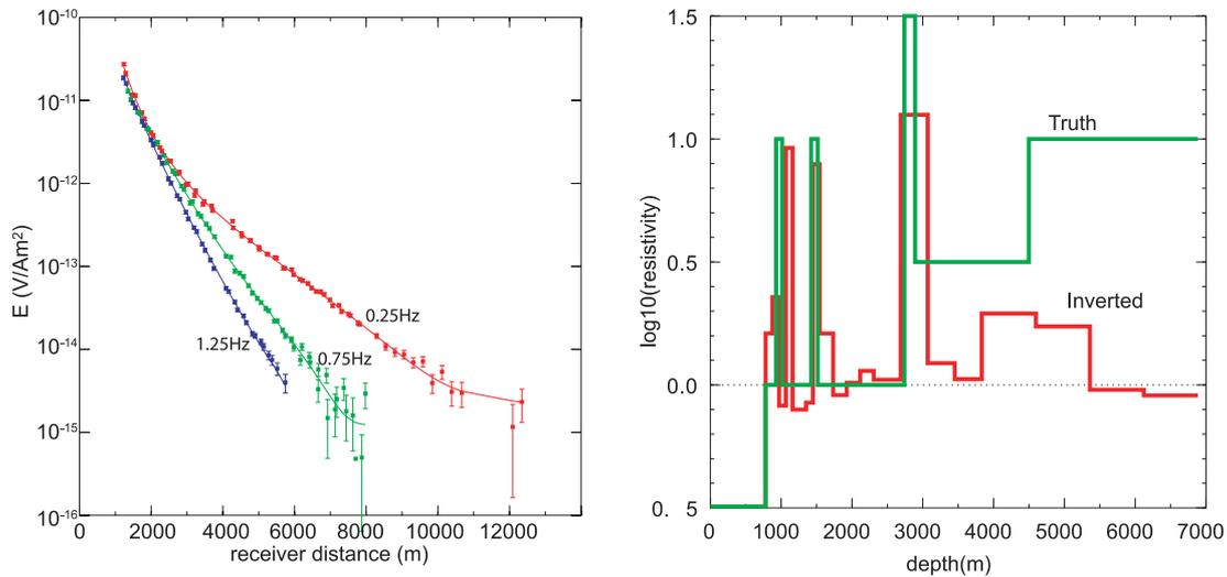
Figure 1: Left; Typical 3-frequency CMP amplitude data used for CSEM inversion, with fitted responses. Right: inversion using meta-parameters for smoothing a finer grid (red curve), compared to green curve truth case.
