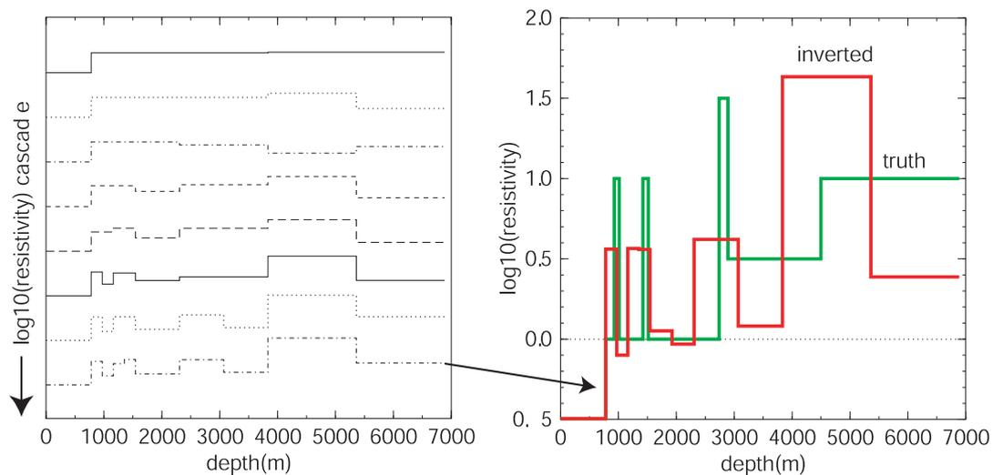
Figure 2: Left; Bayesian model-selection cascade of models used to determine vertical resolution. Algorithm terminates at the lowest model. Right: inverted model (red) against known truth case (green).
