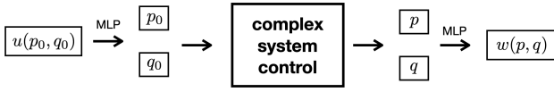
FIG. 15. Diagram of how to include input variables u(p, q) (which includes control functions) and output variables w(p, q) into the control system workflow. MLP is a Multi Layer Perceptron.
