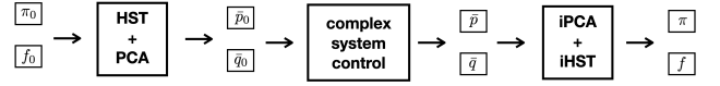
FIG. 16. Diagram of how the Heisenberg Scattering Theory (HST) and a Principle Components Analysis projection (PCA) are incorporated into the complex control system workflow. The inverses are indicated as iHST and iPCA, respectively.
