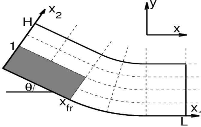
Fig. 1. Schematic of the coordinate system used in the simulations. The angle  $\theta$  between the  $x_1$ -axis and the horizontal is allowed to vary with  $x_1$  to model varying slopes. The dark region corresponds to the initial position of heavy fluid and is constrained by  $0 \leq x_1 \leq x_{fr}$ ,  $0 \leq x_2 \leq 1$ . The height and length of the computational domain are  $H$  and  $L$ , respectively.
